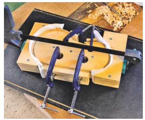
...that was designed to accommodate eight 1.5mm veneers cut from beech
